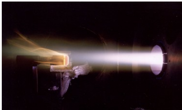
Fig. X. Test of ablative material in the VKI Plasmatron facility
